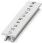
Zack marker strip, Strip, white, labeled, horizontal: L1, L2, L3, N, PE, L1, L2, L3, N, PE, mounting type: snap into tall marker groove, for terminal block width: 5.2 mm, lettering field size: 5.15 x 10.5 mm, Number of individual labels: 10
