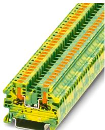
Ground modular terminal block, number of connections: 2, connection method: Push-in connection, 1 level, Rated cross section: 2.5 mm<sup>2</sup>, cross section: 0.14 mm<sup>2</sup> - 4 mm<sup>2</sup>, mounting type: NS 35/7,5, NS 35/15, color: green-yellow
